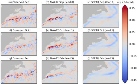
Figure 14. Observed linear geostrophic current speed trends from the AVISO satellite altimetry product in September, October, and February (a, d, g), and speed trends in September-initialized forecasts that verify in the same months from the NWA12 model (b, e, h) and the SPEAR model (c, f, i).
